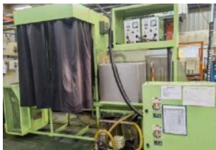
Magnetic Particle Inspection for surface crack verification
