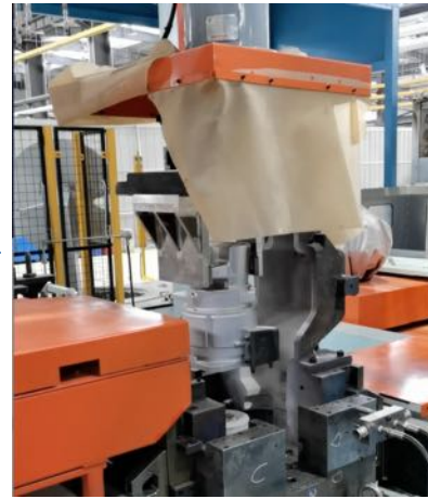
Die opening and extraction of the part
