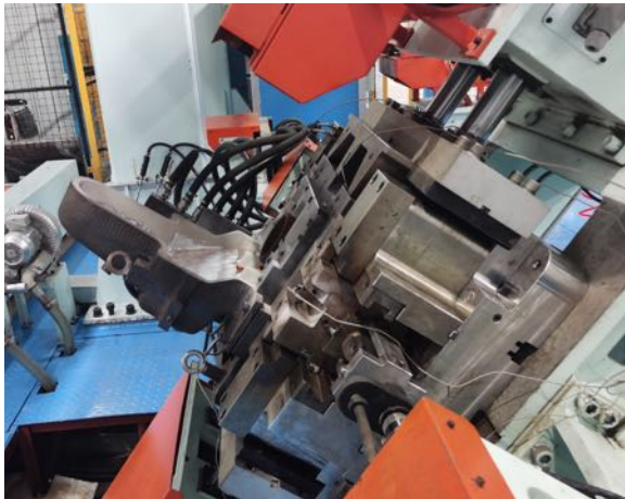
Mould rotation to minimise turbulence during filling
